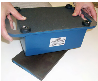
Above: Model D-3 used in inverted position to demagnetize a surface plate.
