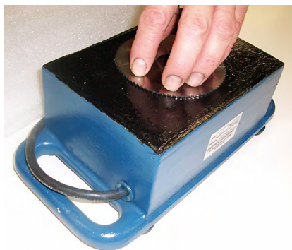
Above: Object to be demagnetized is drawn slowly across surface.
