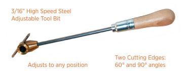
For removing fins of mica and burs of copper from the edges of commutator bars after undercutting with a U-shaped saw.
