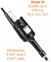
Model 10Model 10 is ideal for full-shift<br/>duty in the tool room or in<br/>production bench grinding,<br/>de-burring, etc. It is forced-<br/>air cooled, and two precision<br/>bearings in steel seats assure<br/>positive rigidity. Model 10 uses<br/>high-speed steel or carbide burs<br/>up to 3/8" diam., or mounted<br/>wheels up to 1" diam. Has 1/4"<br/>collet and 1/8" reducing sleeve.
