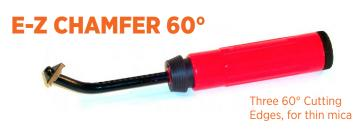
Special ground, 3 cornered insert, chamfers copper on both sides of commutator slots after undercutting. Tool is originally supplied with a H.S.S. insert. An optional Carbide replacement insert is available.
