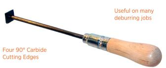
Specially ground 4 cornered carbide insert chamfers copper on both sides of commutator slots after undercutting. Flat sides of the insert can be used for scraping, deburring and chamfering corners on many parts. When insert is dull on all cutting edges, it is easily replaced.
