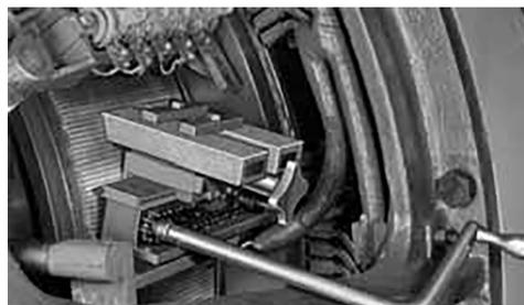
Grinder mounted on a Dieselelectric Generator
