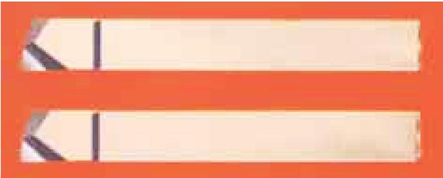
Diamond tipped turning tools shown are used in the finishing of the commutator surface. Steep rake angles on the tool ensure clean cutting of the copper, leaving no smearing or drag over across the mica. The nose radius of .010" leaves a very smooth surface to the copper requiring minimal preparation for the seating of brushes.
