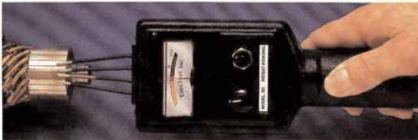
Figure 2 Circuit shorted (red probe indicates location)
