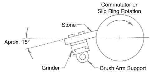
resurfacers trail at 15 degrees off perpendicular in relation to the commutator face, in the direction of machine rotation. The grinder is mounted parallel to the axis of the generator or motor, and to the face of the commutator (unless tapered), and as close as possible.
