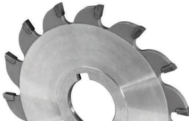
Carbide Tipped saw after retipping and reshaping in optimum condition.
