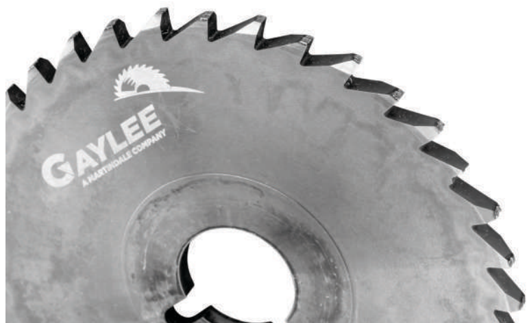
Solid carbide saw with dull, worn teeth.
