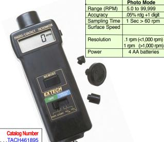
Model 461895 Tachometer with accessories and case ....TACH461895 Net Weight with accessories & case 1 Lb. 10 oz., Shipping Weight 3 Lbs.
