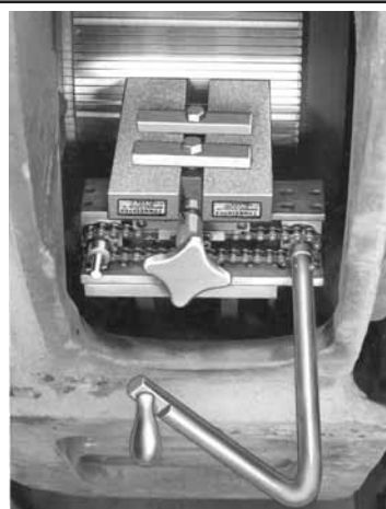
Grinder mounted on Traction Motor
